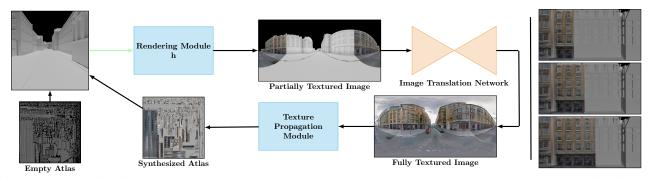
Figure 2: At each iteration our system creates a *partially textured image* by rendering the 3D geometry(top left) using the *synthesized atlas* containing texture from previous iterations. Mesh parts that have not been textured so far are rendered in grayscale. The *texture propagation module* uses the generated image to update the texture atlas used in the next iteration. A visualization of our iterative texturing synthesis output is displayed on a characteristic building facade on the right.
