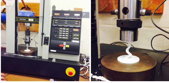
Figure 10: Photographs showing the Instron Universal Testing machine, which applies increasing axial force on the shape until it breaks.
