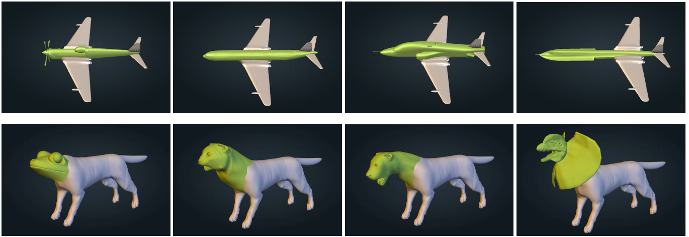
Figure 2: Exploration with semantic attributes for 3D modeling. Top: Exploring less (left) to more (right) aerodynamic fuselages. Bottom: Exploring less (left) to more (right) scary heads. The adjectives “aerodynamic” and “scary,” and the ranking of components under these attributes were learned from crowdsourced training data. The displayed components, left to right, have \sim 0\% , 33\% , 66\% and 100\% of the respective attribute strengths. All components are automatically positioned and glued.
